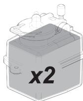
After the first tank, drive the car in a circle at half throttle for two tanks of fuel.
