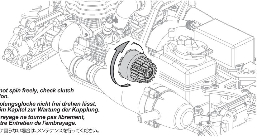
**!** If clutchbell does not spin freely, check clutch maintenance section.
