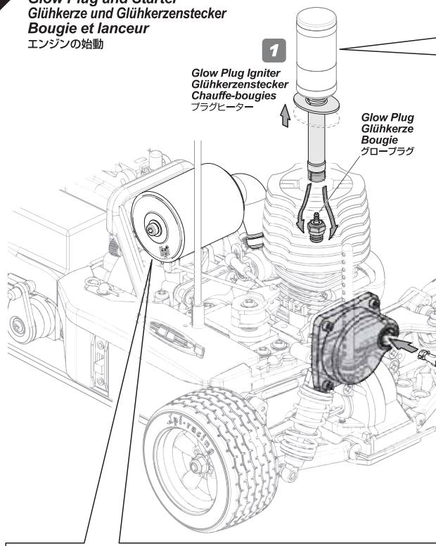
Attach the glow igniter to the glow plug. Start the engine by cranking with the Roto Start. Remove the glow igniter as soon as the engine is running. If the glow plug igniter is left connected while the engine is running, it will drain the battery and damage the glow plug.
