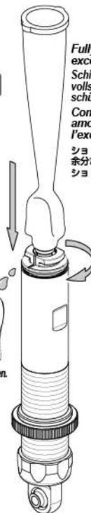
Fully compress shock to bleed excess oil before tightening.
