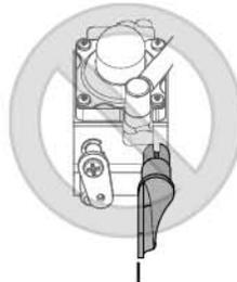
Choke lever should not be in this position.
