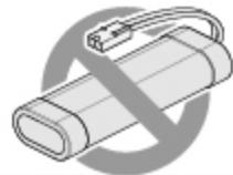
**Do not use NiCd/NiMH battery chargers for LiPO batteries.** If you do not use a special charger for LiPO batteries, they will be damaged. When using 3S LiPo packs, cell quality is very important. We recommend battery packs with a 25C rating or better. Using batteries with a lower C rating may result in damage to your batteries.
