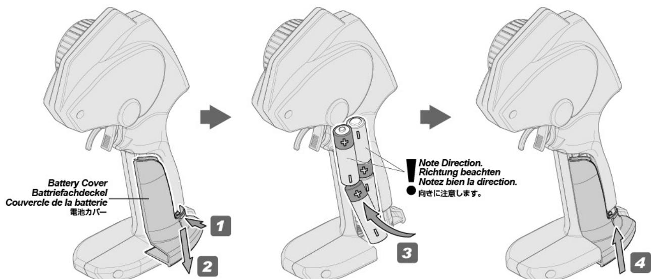
**Open battery cover at the bottom of transmitter. Install batteries. Follow the direction of batteries designated in the inside of battery box.**
