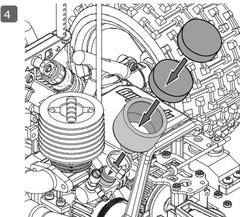
Drain all remaining fuel from the fuel tank. Use a fully charged glow igniter and try to restart the engine to burn any remaining fuel out of the lines. After burning off the fuel, remove the glow plug and add several drops of after run oil, then crank the engine over to spread it throughout the engine.
