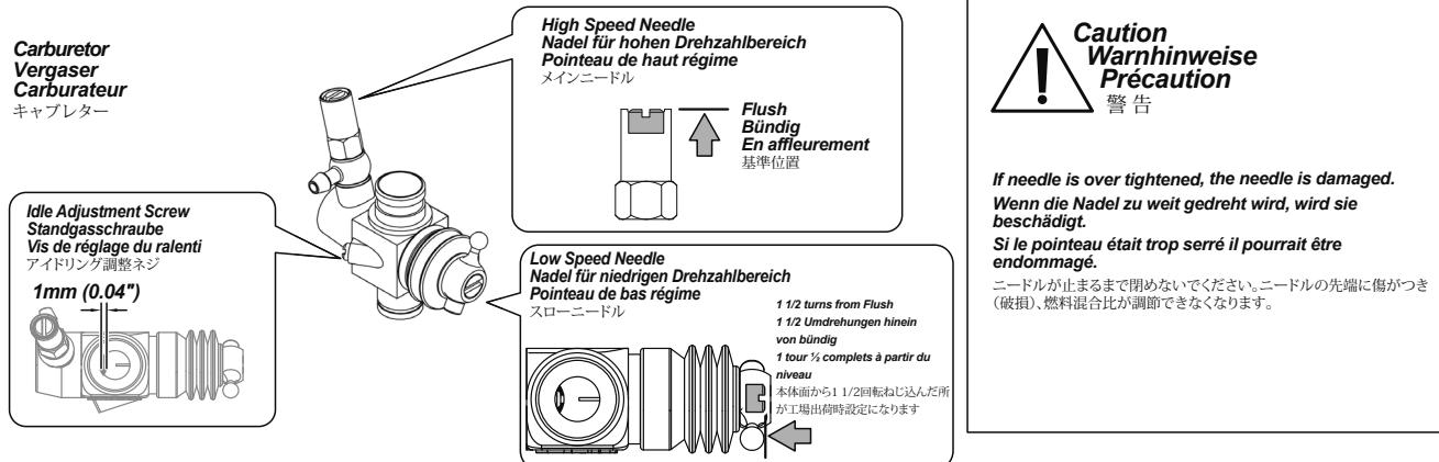
These are the factory settings for the High Speed Needle and Low Speed Needle and are ideal for breaking in and starting your engine. Resetting the carburetor to the Factory Break In Settings is always a good starting point if retuning your engine
